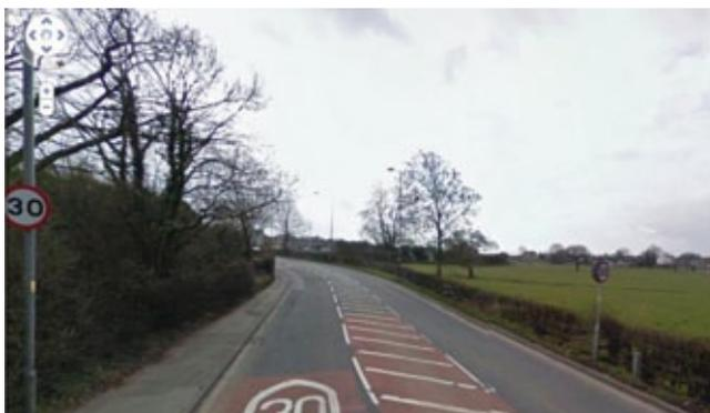
**Figure A2.3: High-speed section with unprotected poles at the edge of the carriageway**
